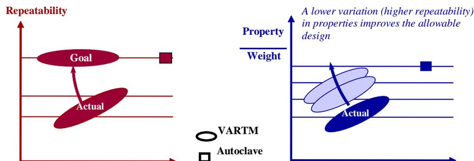
Figure 1: VARTM has the potential to reduce cost with equivalent repeatability compared to autoclave processing
