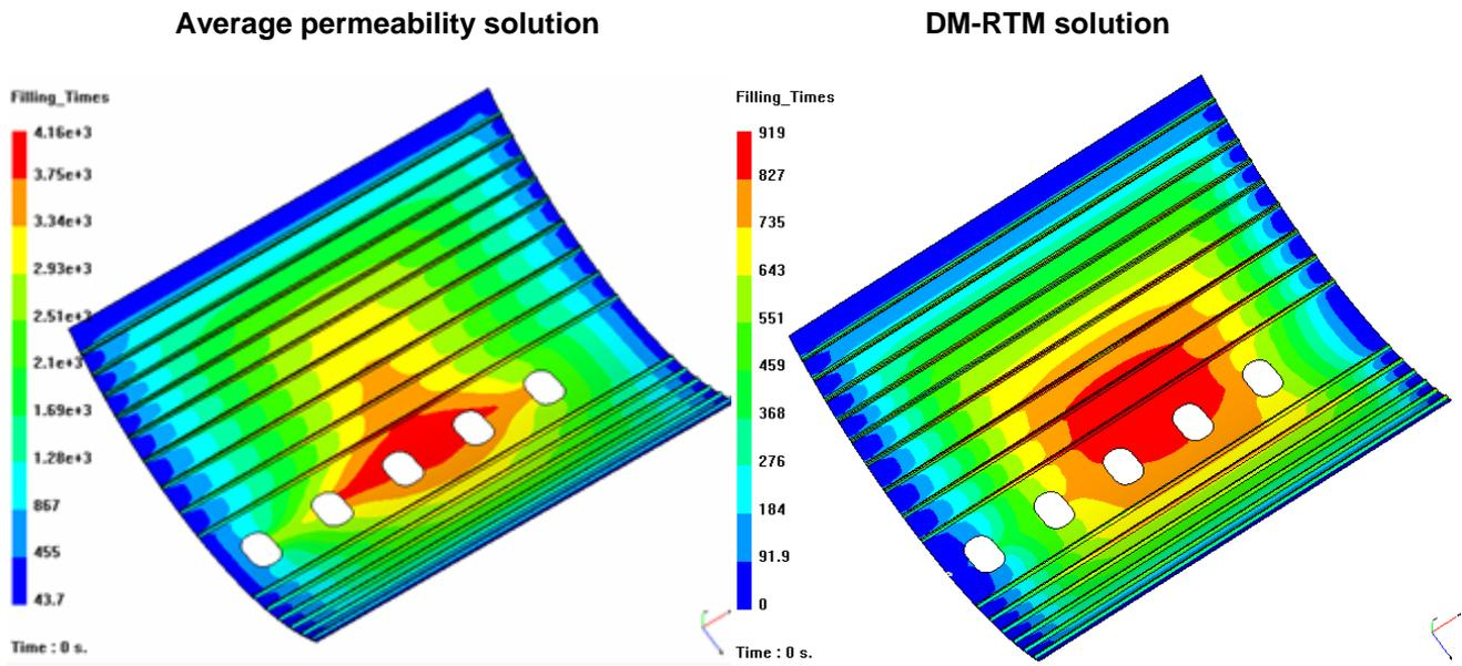
Figure 9. Comparison between the average solution and the proposed DM-RTM solution.
