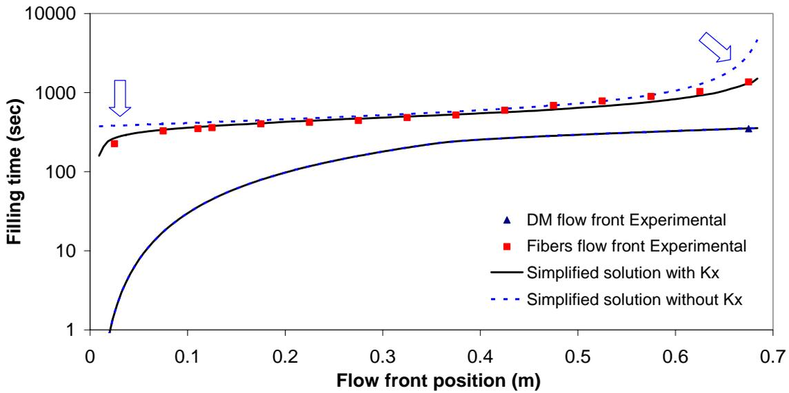
Figure 7. Experimental validation of the proposed simplified approach to simulate DM-RTM mold filling.
