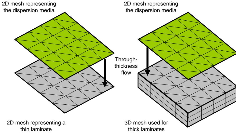
Figure 3. Two proposed geometrical representations: a 2D FE mesh is used to describe thin laminates (i.e., for shell-like composites) and a 3D FE mesh is used in the case of thick composites. In both cases a 2-dimensional FE mesh is used to describe the DM.
