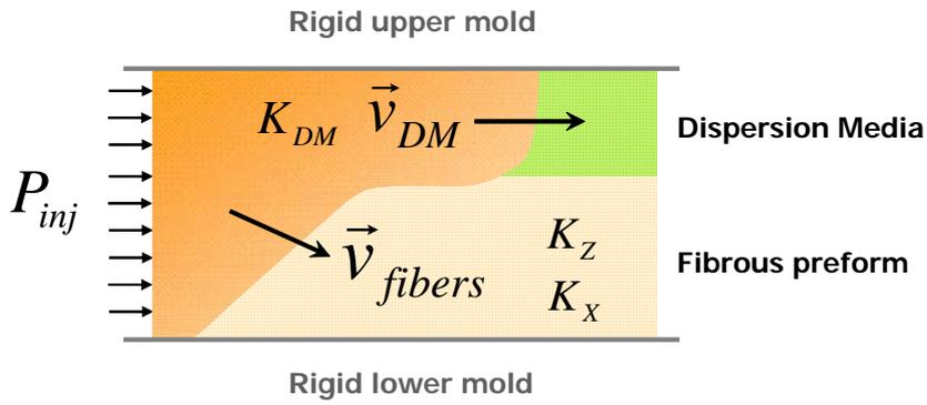
Figure 1. DM-RTM manufacturing process: a highly permeable dispersion medium is added above the fibrous preform to facilitate resin impregnation.
