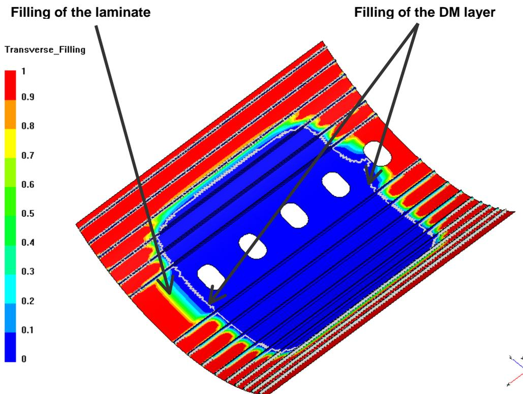
Figure 10. DM-RTM filling simulation of an aeronautical test part: in-plane filling of the DM layer and transverse flow through the laminate can be observed.
