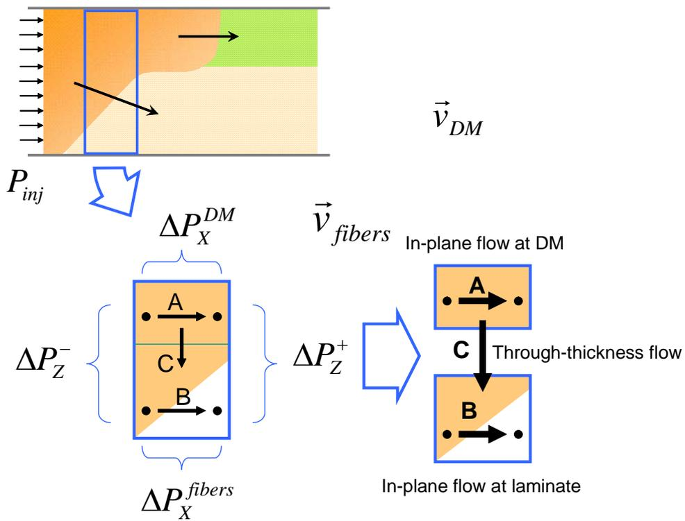
Figure 2. Pressure and resin flow distribution during DM-RTM mold filling.
