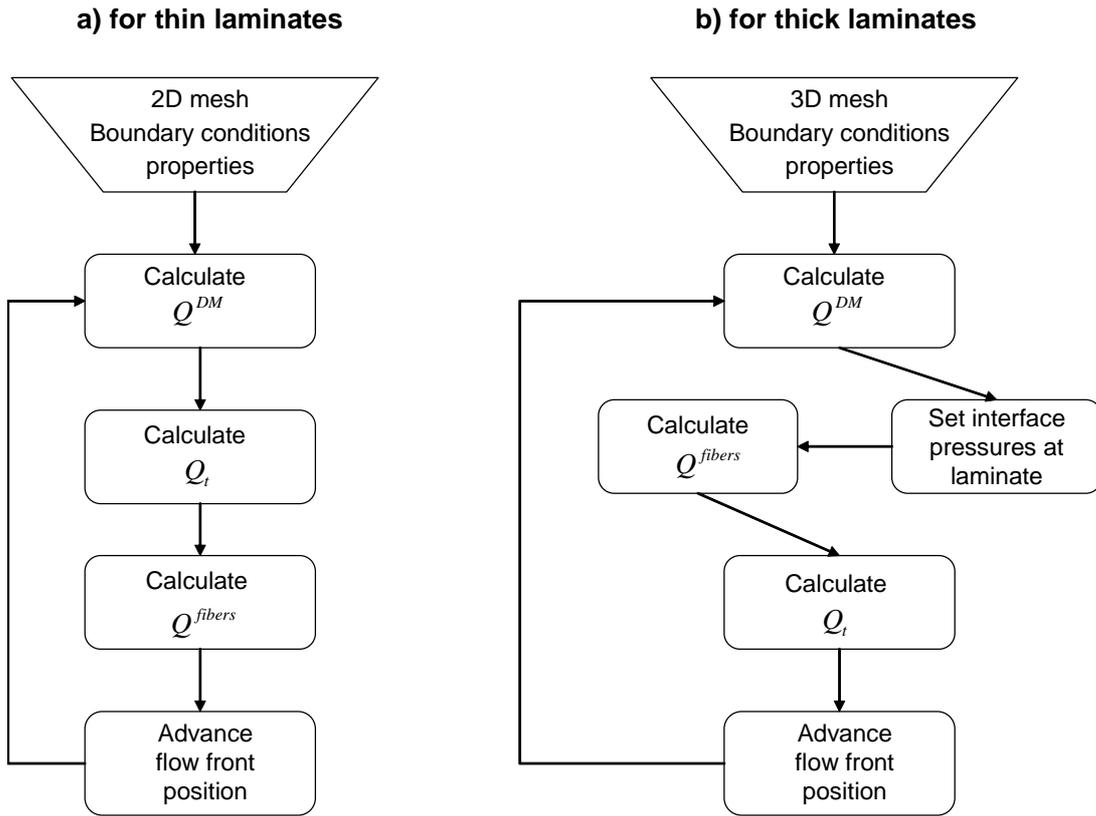
Figure 5. Flow chart of the finite element solver used to simulate DM-RTM mold filling for thin and thick laminates respectively.
