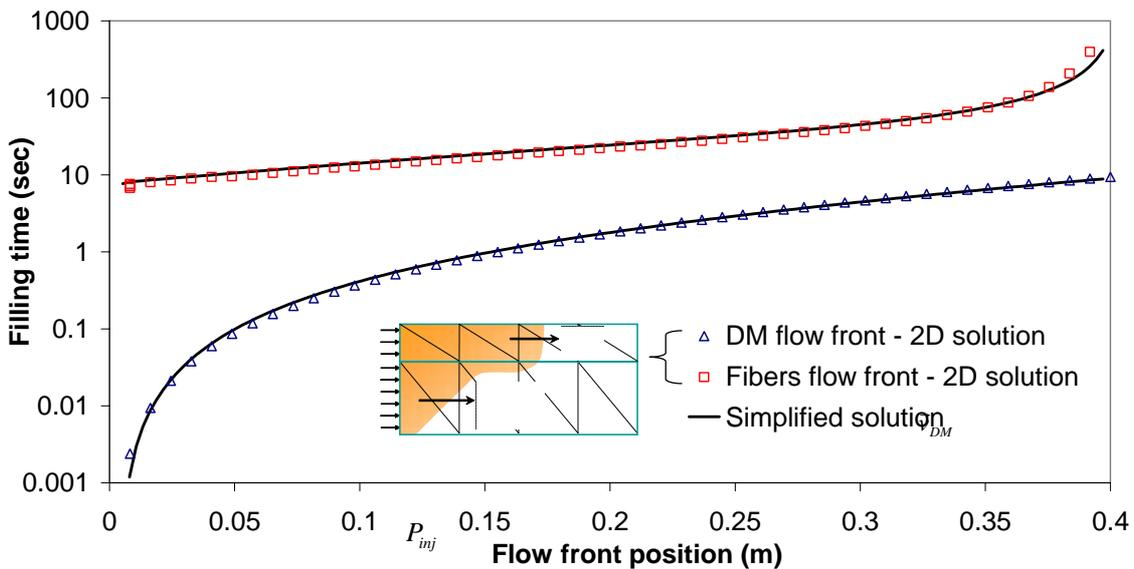
Figure 6. Comparison of the proposed simplified DM-RTM solution with a 2D through-thickness FE solution.
