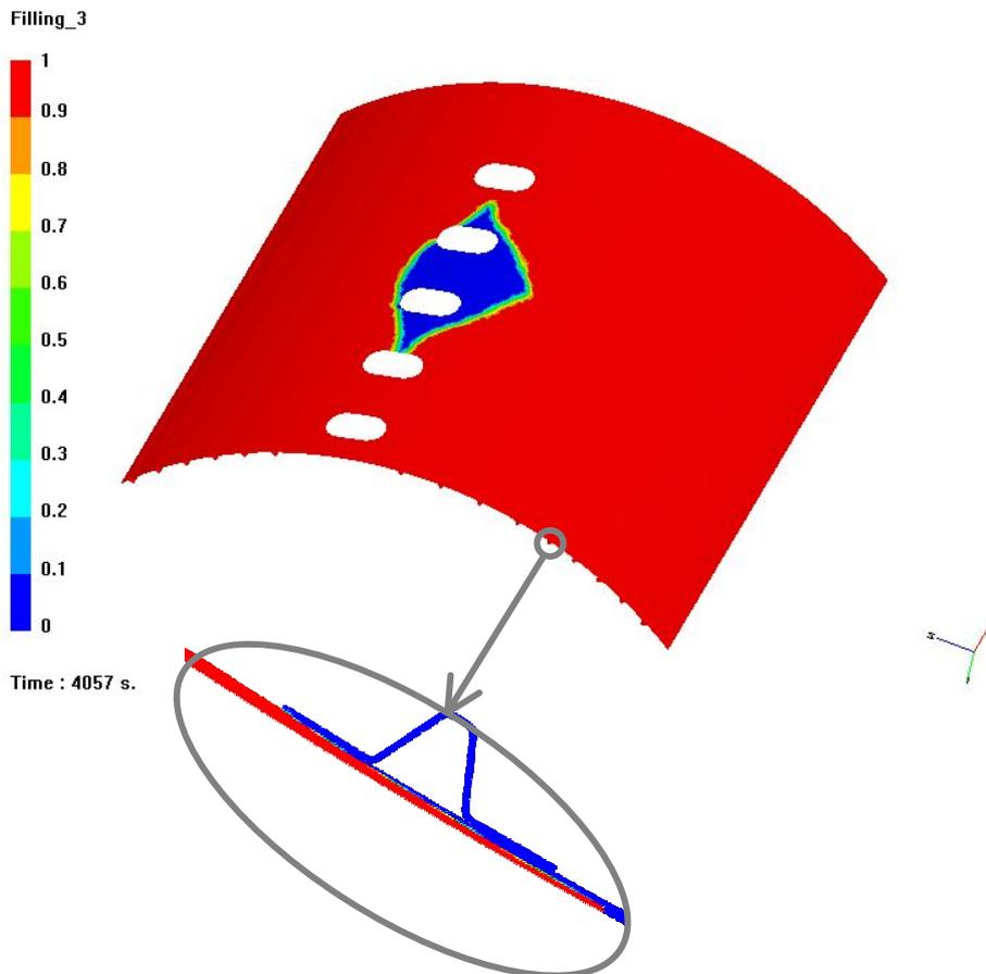
Figure 8. Filling results of the aeronautical composite part with the average permeability solution for a mesh of shell elements.
