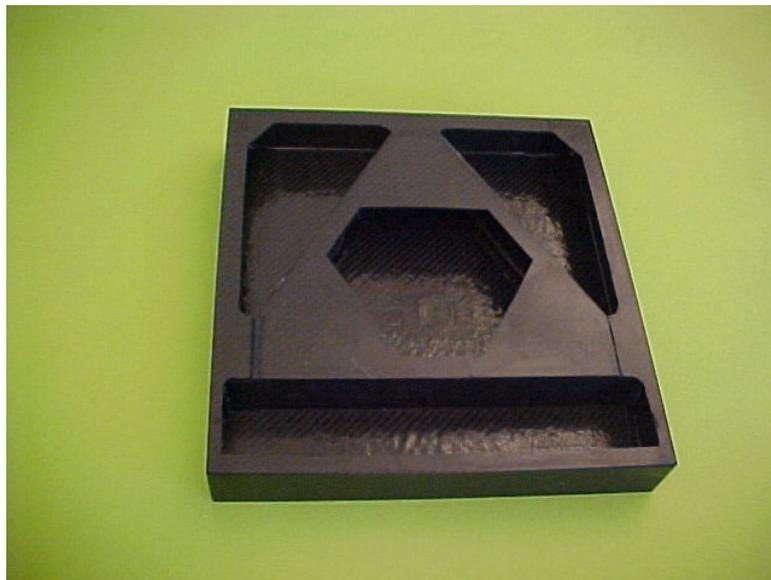
Figure 5: The assembled carbon carrier structure
