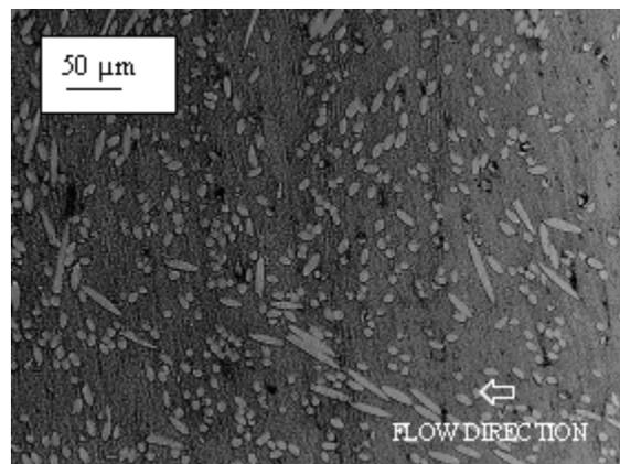
c. Higher degree of out of plane orientation of fibers at location  $A_{ii}$  (Case III)
