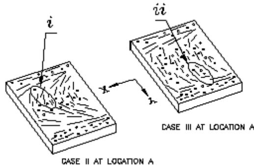
a. Schematic pattern of fiber orientation at location A (Cases II & III)
