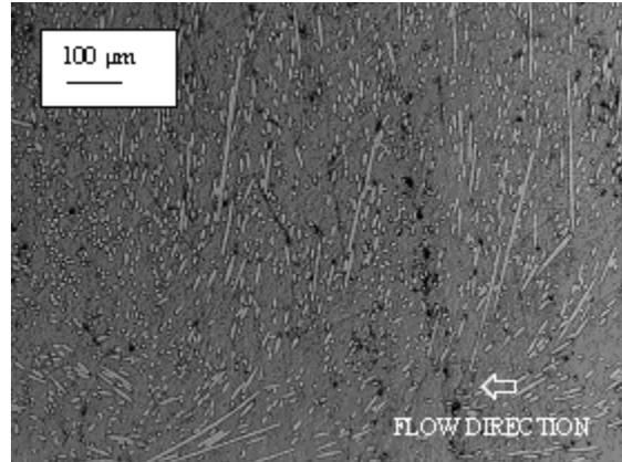
c. Higher degree of transverse orientation of fibers at location B (Case III)
