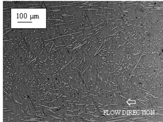
b. Lower degree of transverse orientation of fibers at location B (Case II)
