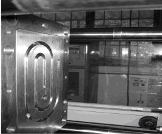
a. Spiral mold cavity plate
