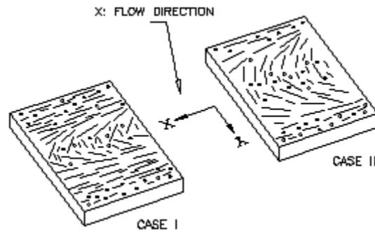
a. Schematic pattern of fiber orientation at location A (Cases I & II)
