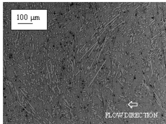
c. Higher degree of transverse orientation of fibers at the centerline (Case II)
