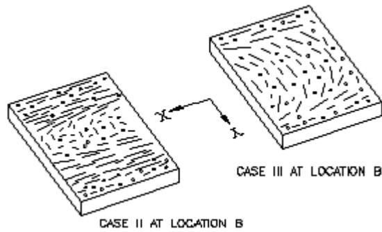
a. Schematic pattern of fiber orientation at location B (Case II & III)
