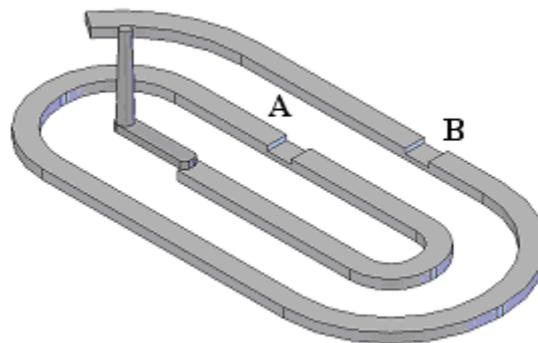
Fig. 2. Cut-sections parallel to the plane of flow at locations A & B for analyzing the state of fiber orientation in the mid-plane (Core layer)
