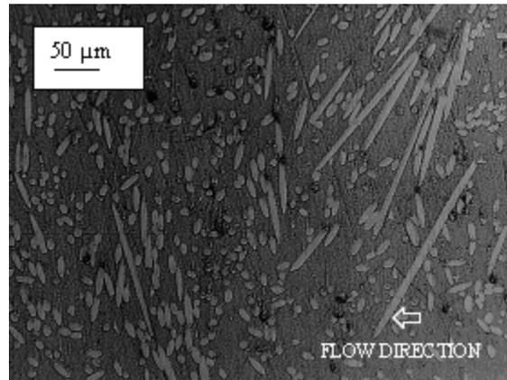
b. Higher degree of in-plane transverse orientation of fibers at location  $A_i$  (Case II)
