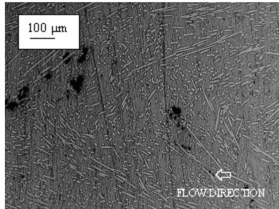
b. Lower degree of transverse orientation of fibers at the centerline (Case I)
