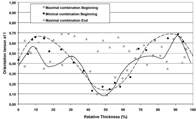
Fig.5: Fibre orientation profiles through-the-thickness of the injection moulded part
