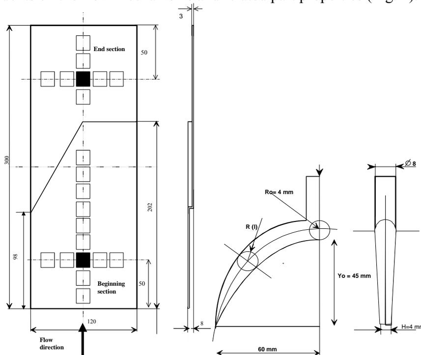
Fig.1: Plastic part and fan gate geometry and cutting pattern of test samples for fibre content (white coupons) and fibre length and orientation (black coupons) determination
