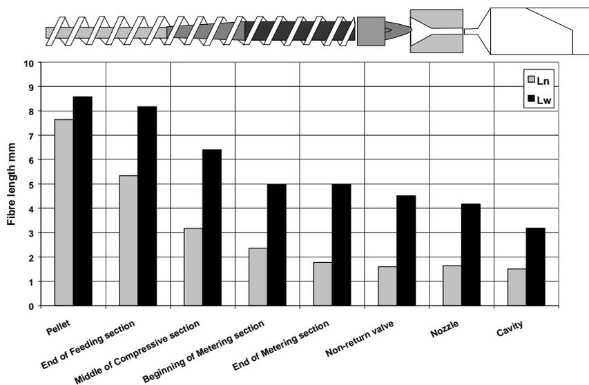
Fig.4: Number- and weight-average fibre lengths along the processing system
