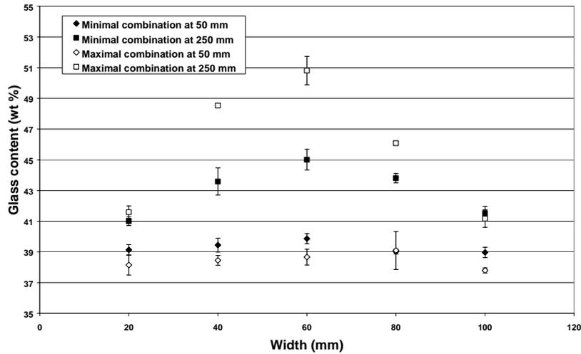
Fig.3: Glass weight content along the width of the composite plates.
