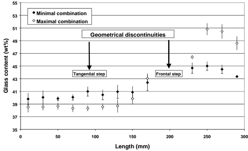
Fig.2: Glass weight content along the mid-axis of the composite plates
