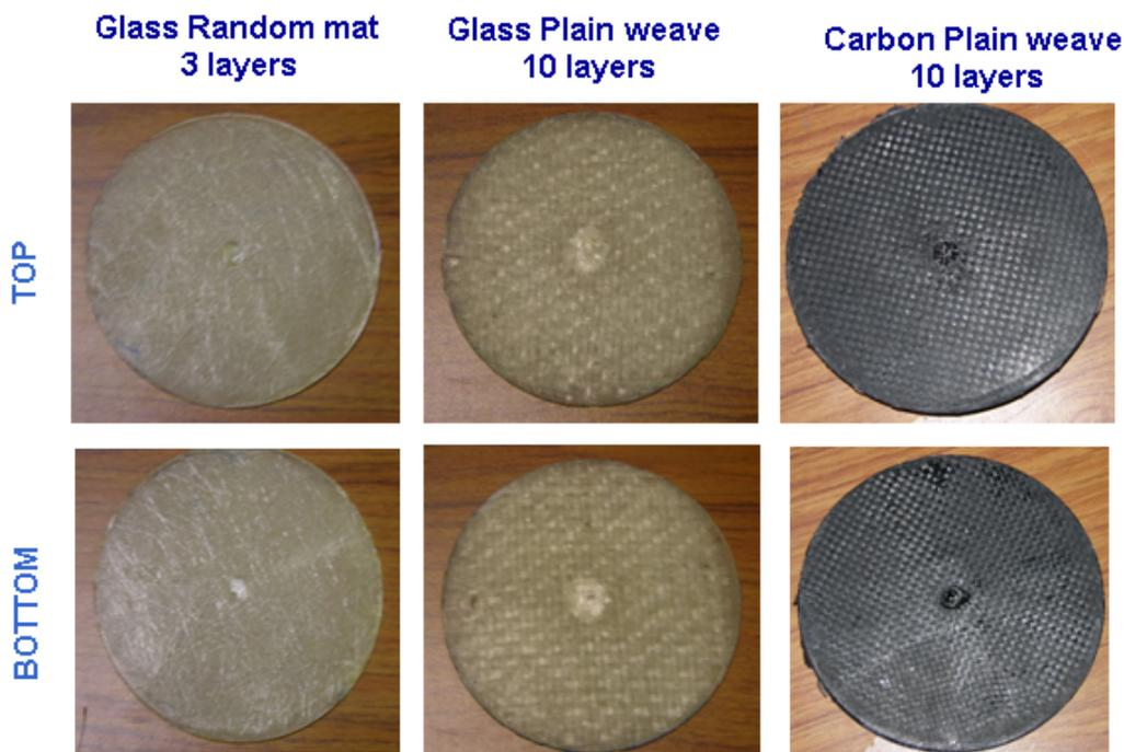
Figure 7: Examples of manufactured parts with the new low cost Compression RTM press
