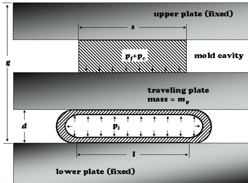
Figure 2: The internal pressure of the hose counteracts the weight of the traveling plate, the compaction pressure of the fabric, and the fluid pressure of the resin.
