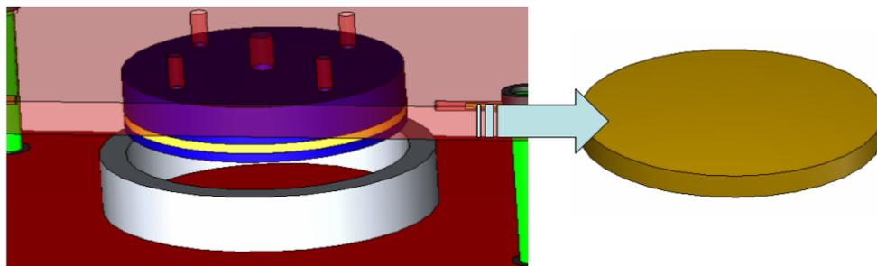
Figure 6: The mold was designed to manufacture circular disks to facilitate in the operation of the press
