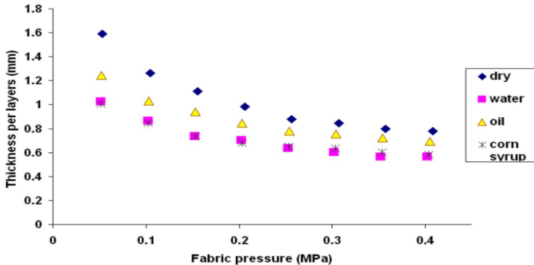
Figure 5: Thickness per layer versus fabric pressure for random mat glass. The viscosity of oil is 54 cps and the viscosity of corn syrup is 146 cps.
