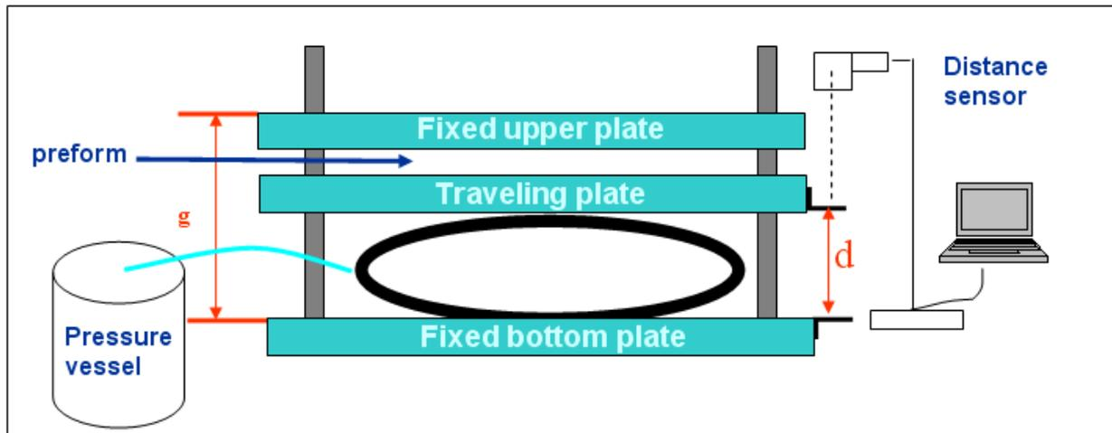
Figure 3: Schematic representation of set-up used for compaction tests
