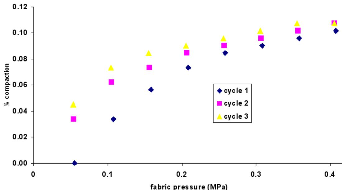
Figure 4: Percent compaction as a function of compaction pressure for three consecutive compressions performed on the same sample of random mat glass
