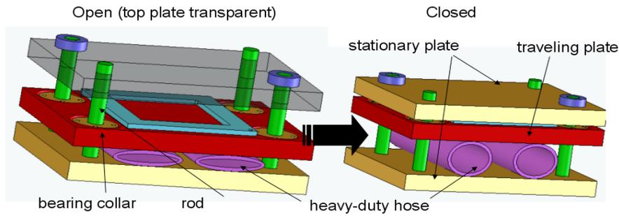
Figure 1: The inflation of a heavy-duty hose between two platens will generate the clamping of the press
