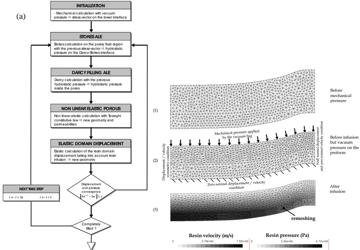
Fig. 6 Resin Film Infusion (RFI) of a curved panel – (a) proposed algorithm – (b) results at initial time (1), compression time (2), final stage (3)
