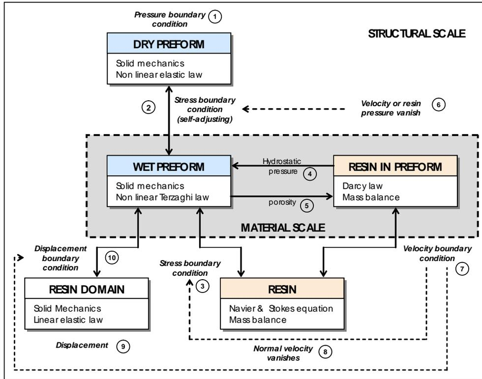
Fig. 3 Boundary conditions at structural scale and interaction at material scale
