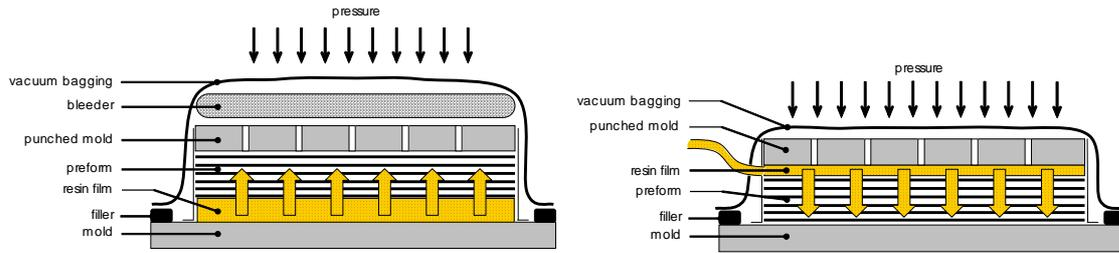
Fig. 1 Composite manufacturing processes by infusion – RFI (a) – LRI (b)
