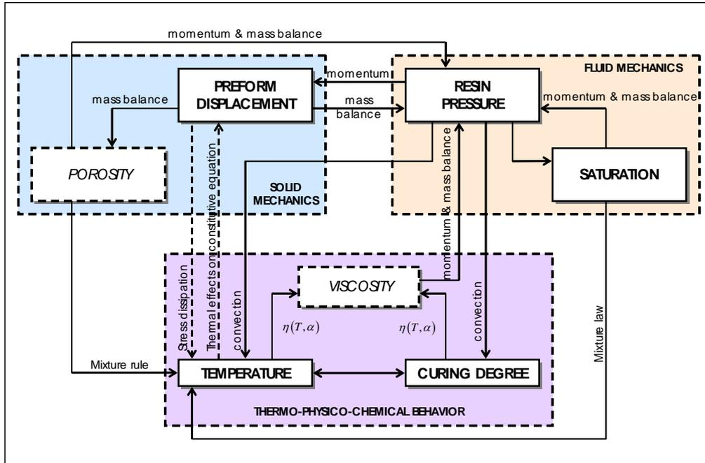
Fig. 4 Coupling between thermo-chemical, fluid and solid mechanical behavior
