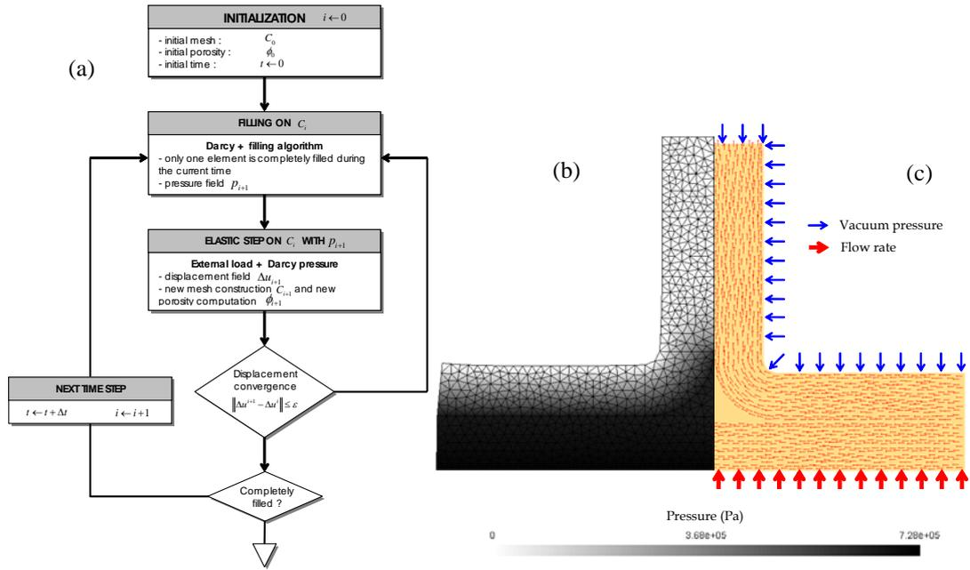
Fig. 5 Infusion of a T: (a) algorithm used - (b) pressure distribution (Pa) on the deformed configuration - (c) permeability orientation for the underformed configuration
