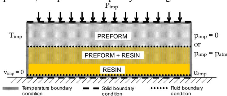
Fig. 2 Composite manufacturing processes by infusion – RFI (a) – LRI (b)
