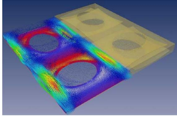
Fig. 15 Resin flow in a glass plain weave
