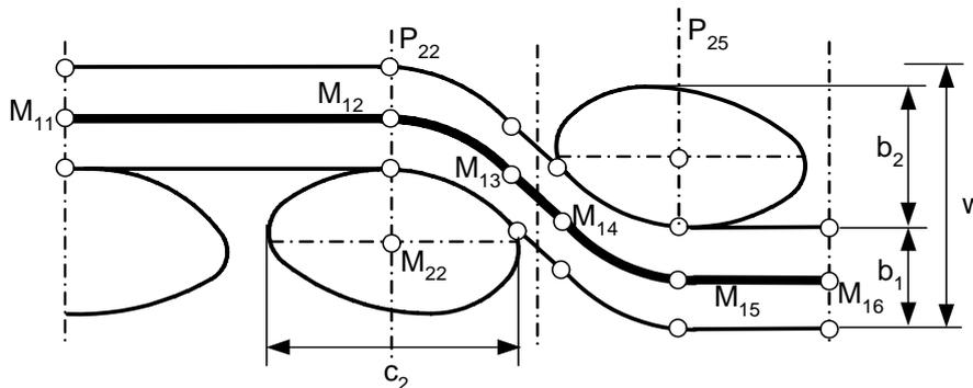
Fig. 9. Transverse cut in the direction 1 of the simplified model for a twill  $m*n$ .
