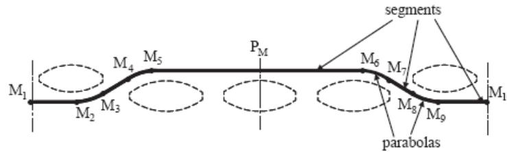
Fig. 8 Model of a trajectory for twill 3 \*2.
