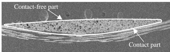
Fig.1 Transverse cut of a glass plain weave. Definition of yarn section
