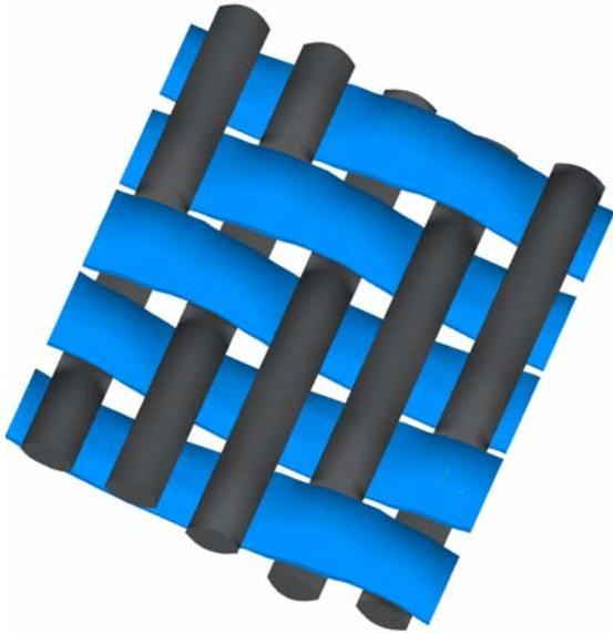
Fig. 10 3D model of a carbon twill 3\*2
