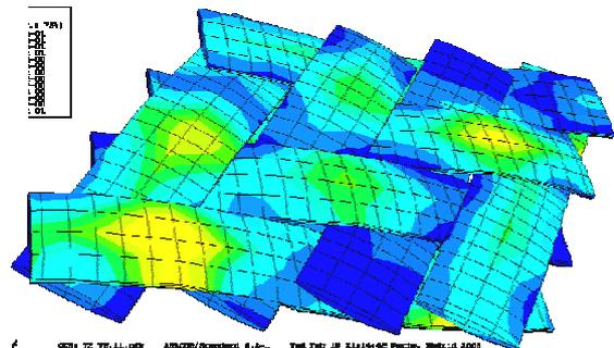
Fig 13 Finite element simulation of the shear deformation of a twill 2\*2
