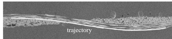
Fig 2 Transverse cut of a glass plain weave. Definition of the trajectory
