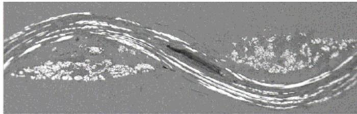
Fig 5 Transverse cut of a Twintex fabric
