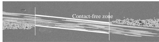
Fig 4 Transverse cut of a glass plain weave, contact free zone
