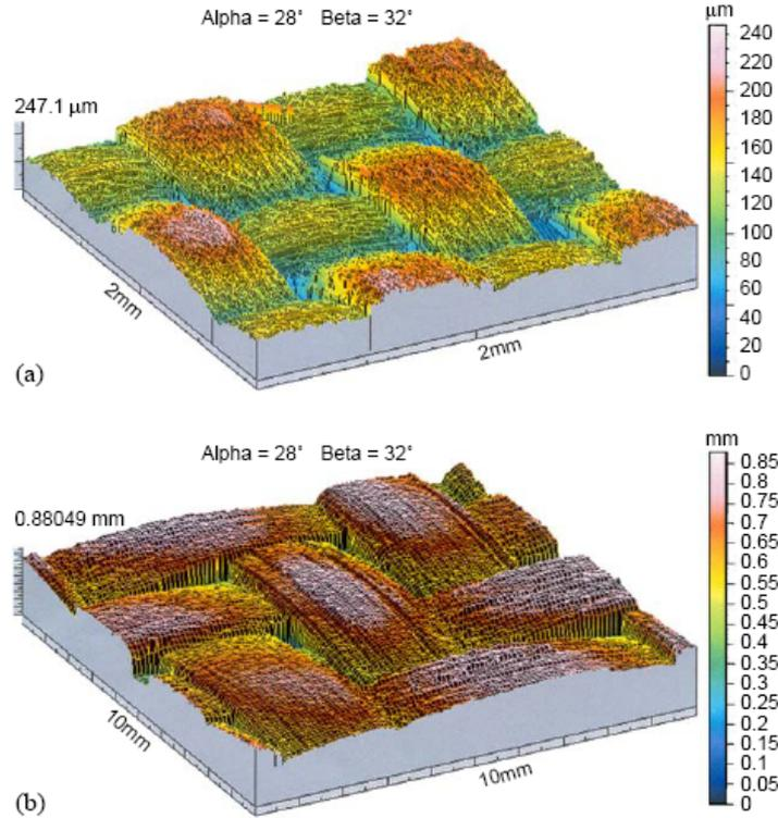
Fig 6. 3D optical measure of dry fabrics at the initial state
