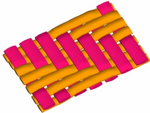
Fig 11 3D model of a carbon twill 4\*3
