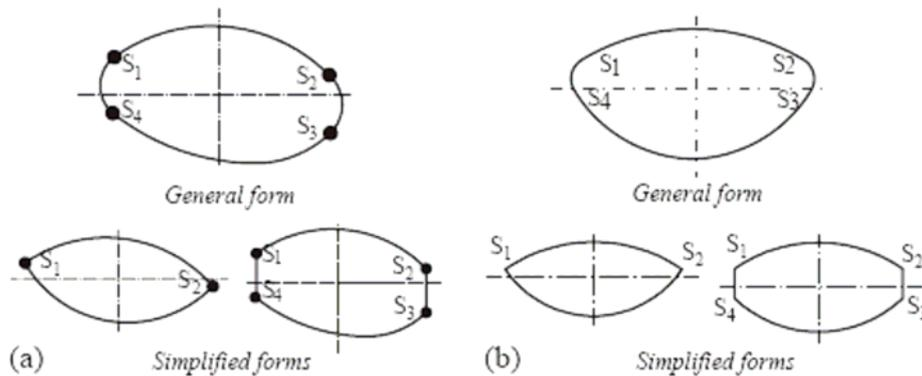
Fig 7. Models for the cross section of a 2D fabric: (a) generic (b) plain weave.
