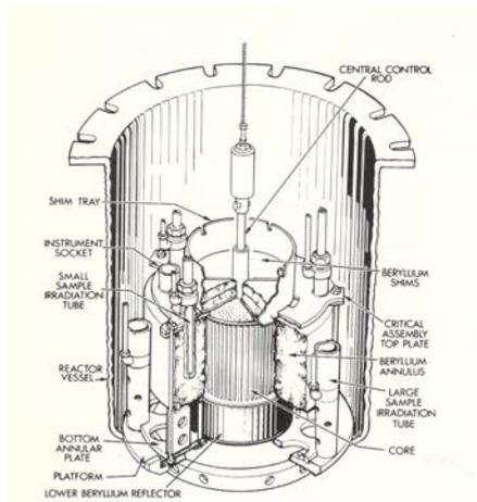
**Fig 1.** Schematic diagram of SLOWPOKE-2 nuclear reactor.
