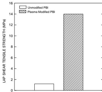
**Fig 7.** Lap shear tensile strength of adhesive joint of surface modified polybenzimidazole.
