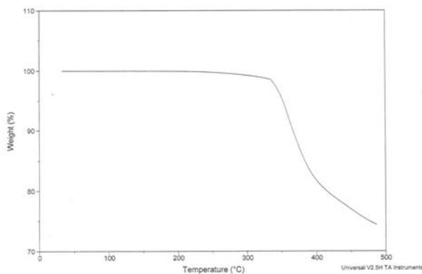
**Fig 6.** TGA plot of the high temperature resistant epoxy adhesive when silicate nano powder dispersed in to the adhesive in 10% weight ratio.
