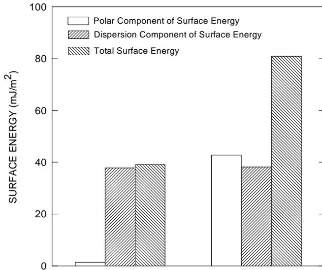
**Figure 4.** Polar, dispersion and total surface energy of polybenzimidazole when the polymer surface is modified by low-pressure plasma.
