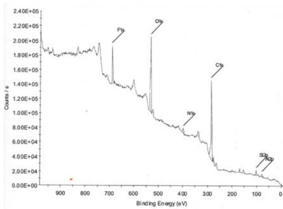
**Fig 2.** ESCA widescan spectra of unexposed polybenzimidazole surface.
