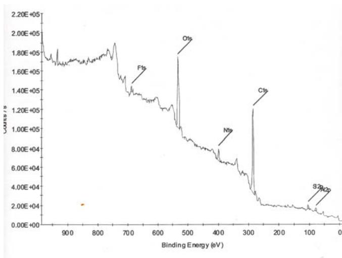
**Fig 3.** ESCA widescan spectra of polybenzimidazole surface modified by low pressure plasma.
