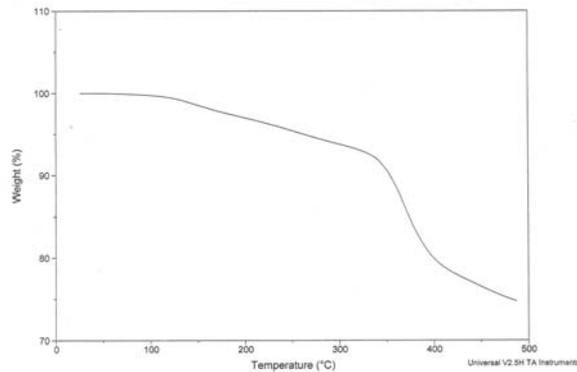
**Fig 5.** TGA plot of the basic high temperature resistance epoxy adhesive.
