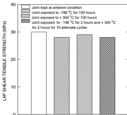
**Fig 9.** Durability under cryogenic, elevated temperature and thermal fatigue conditions of high performance nano silicate epoxy adhesive joint.
