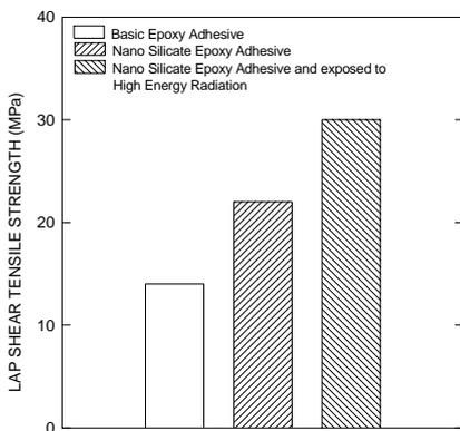
**Fig 8.** Lap shear tensile strength of the joint prepared with basic epoxy adhesive, nano silicate epoxy adhesive and the nano silicate epoxy adhesive joint exposed to SLOWPOKE-2 Nuclear Reactor for 6 hours.
