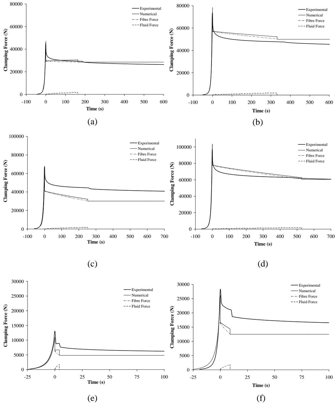
Fig. 5 Comparison of numerical and experimental RTM clamping forces. (a) DMF  $V_f = 0.30$ , (b) DMF  $V_f = 0.4$ , (c) PDF  $V_f = 0.30$ , (d) PDF  $V_f = 0.4$ , (e) CFM  $V_f = 0.30$ , (f) CFM  $V_f = 0.4$
