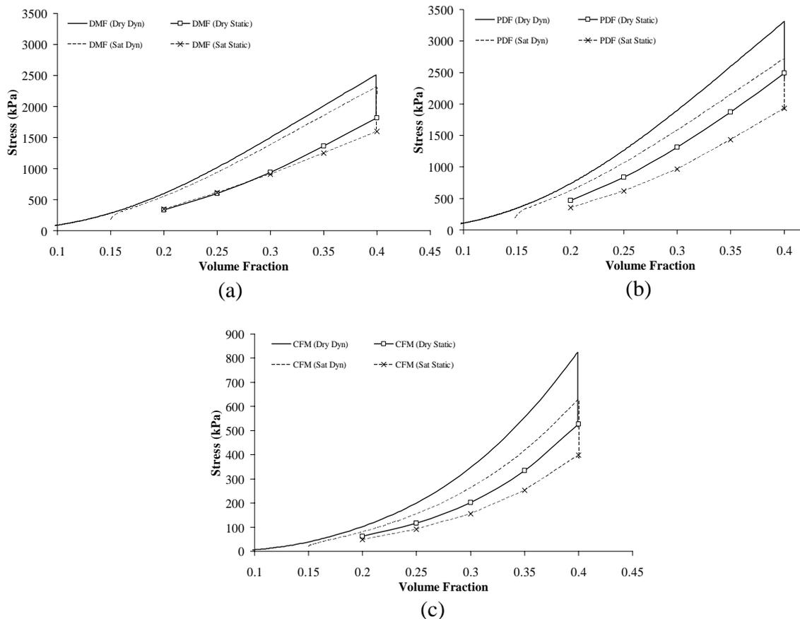
Fig. 3 Dry and saturated dynamic and dry and saturated static compaction response of (a) DMF, (b) PDF and, (c) CFM.
