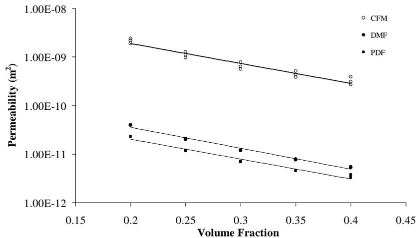
Fig. 4 Permeability comparison between the wood fibre mats and CFM.
