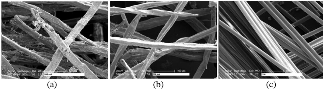
Fig.1 SEM images showing comparison between dry formed, wet formed and glass fibre mats: (a) Dry formed DMF mat, (b) Wet formed PDF mat and, (c) CFM.
