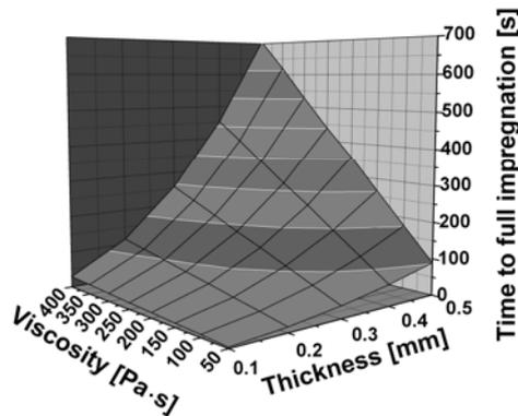
Fig. 7 Time to full impregnation as function of resin viscosity and fibre layer thickness
