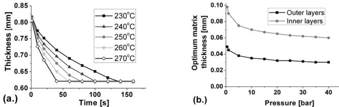
Fig. 6 a) Composite thickness evolution for four 0.2mm fibre layers and constant excess matrix, b) Necessary matrix thickness for outer and inner matrix layers depending on pressure for 0.2mm fibre layer thickness
