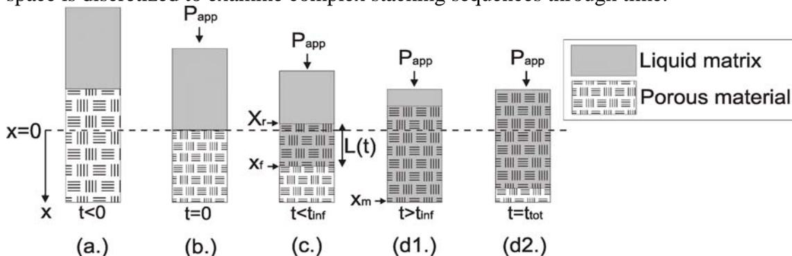
Fig. 1 Stages in the one dimensional infiltration model, after Michaud [4]
