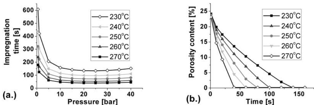
Fig. 8 For 0.2mm fibre layer thickness; a) Time for complete impregnation and b) The porosity content in the composite through process time at 20bar
