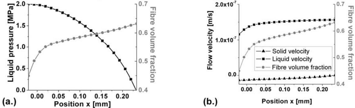
Fig. 2 The results for  $V_f$  together with a) polymer pressure and, b) flow velocities for 20bar applied pressure, 250°C and 75s impregnation time
