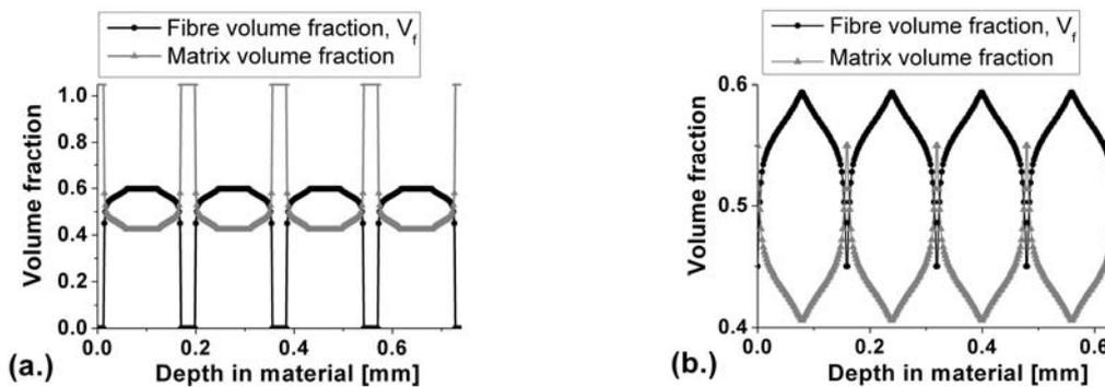
Fig. 3 The results with 4 fibre layers processed at 250°C and 10bar for: a) a partially infiltrated material after 30s and, b) a fully infiltrated material after 100s
