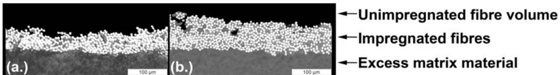
Fig. 4 Impregnation after: a) 15s, and b) 60s by nominally 6bar at 250°C
