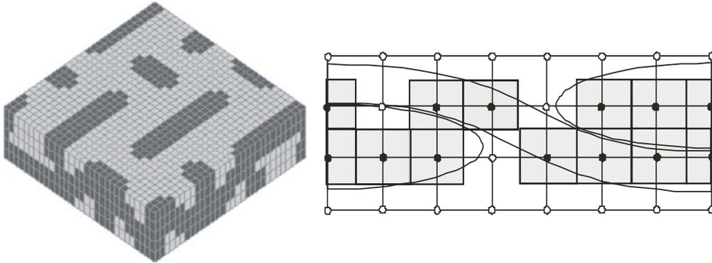
Fig 2 A 3D and 2D voxel representation of a textile geometry
